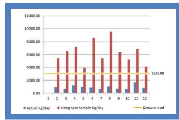
COD peaks at the start of the discharge flow stream but does not continue for the whole period of discharge to sewer.
