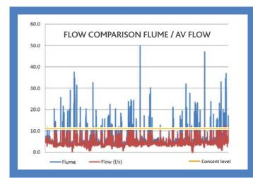
The graph shows a vast, consistent breach of consent when using data from the primary flow measurement, which is not the case when using data from the **MSFM**.
