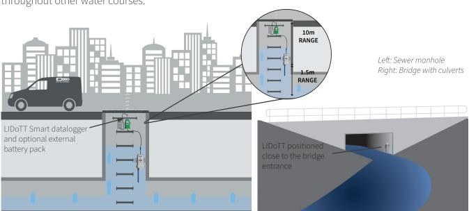
**LIDoTT**<sup>®</sup> is ideal for widespread deployment in sewer networks, in domestic sewer manholes and throughout other water courses.
